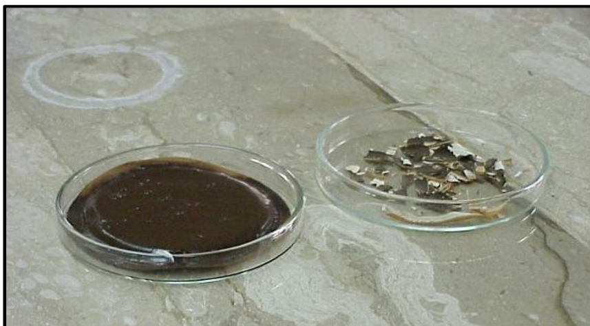
Result with OBM cake : Before and after HDC Mk II treatment for 6 hrs @ 90 °C resulted in 95% dissolution .
