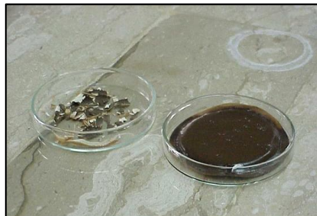
Result with OBM cake: Before (right) and after (left) HDC Mk II treatment for 6 hrs @ 90 °C gave 95% dissolution.
