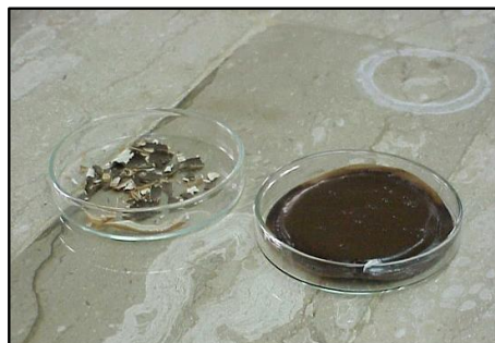
Result with OBM cake: Before (right) and after (left) HDC Mk II treatment for 6 hrs @ 90 °C gave 95% dissolution.
