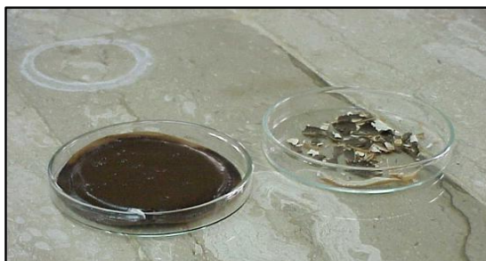
After 6 hours soaking at 90°C, the SBM filter cake is 96% dissolved. Also works in WBM
