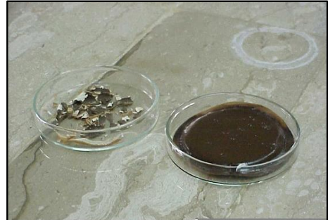
Result with OBM cake: Before (right) and after (left) SD27X treatment for 6 hrs @ 90 °C gave 95% dissolution.
