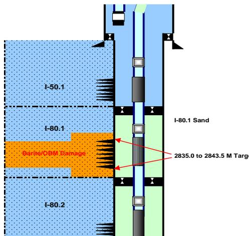
The zone was isolated from the lower production and bull-headed with 3500 liters each of PentaFlow/PowerPickle® (50/50) and HDC MARK II and allowed to soak overnight. The well was gas lifted from the SSD successfully producing 11 mmscfd and building.
