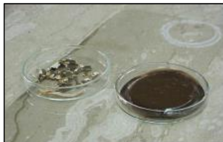
Result with OBM cake: Before (right) and after (left) SD27X treatment for 6 hrs @ 90 °C gave 95% dissolution.
