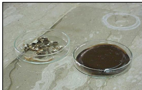
Result with OBM cake: Before (right) and after (left) HDC MK II treatment for 6 hrs @ 90 °C gave 95% dissolution.
