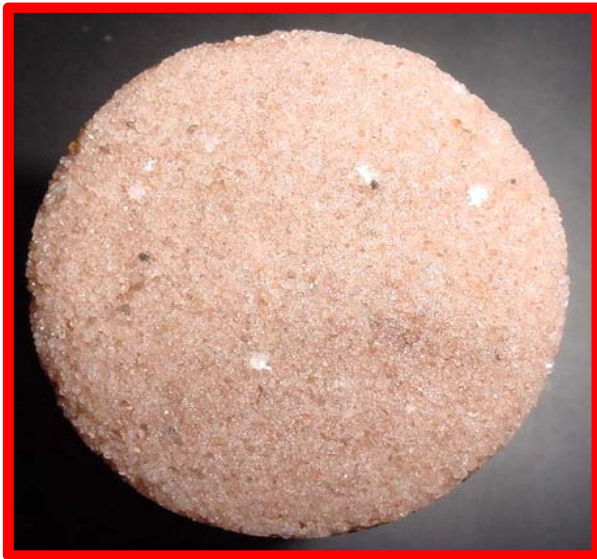
Photo 1. Core inlet before the injection of the drilling mud
