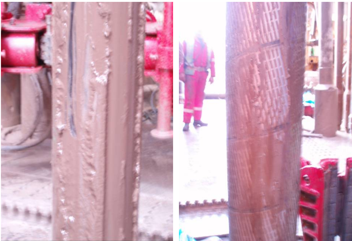
Picture 1: Screens that were pulled out from the aborted 1 st completion run with shroud covered with mud solids. The picture on the left shows one of the lowest screen joints as it was removed from the well. A higher joint shown in the right picture which had not entered into the PDL showed slightly less mud coating but the screen shroud was still blocked.
