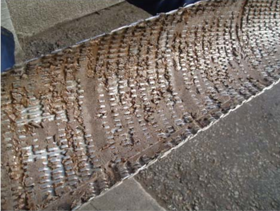
Picture 2: mud coated on inner section of screens shroud from aborted 1 st completion run.
